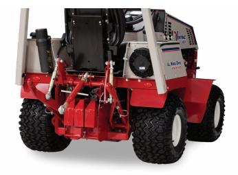
The Category One 3-Point Hitch adds the benefit of using numerous light and medium-duty implements\* on the rear of Ventrac 4000 Series Tractors. An eight-inch stroke hydraulic cylinder lifts up to 750 pounds (340 kg) at the draw bar through a 14 inch (26 cm) lift range. Each draft bar has a fast pin, adjustable stabilizing bar, and adjustable lift linkage.
