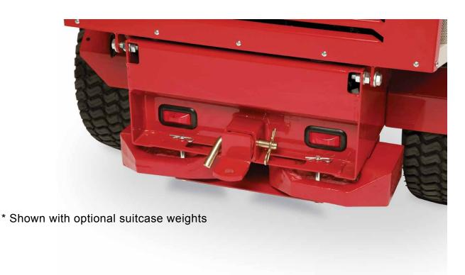
The rear weight bracket is available for adding additional weight to the rear of Ventrac 3100 and 3200 tractors. The tractor may perform better with additional rear weight while operating specific attachments, or working on grades.
