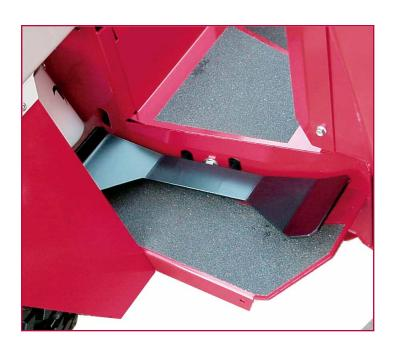
The optional Foot Control Pedal can free your right hand up for forward and reverse motion on the 4000 series. This is necessary for operating the VERSA-loader attachment and helpful when using the optional rear 3-Point Hitch.
