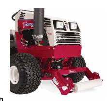
new landscape beds, cutting back sod for new garden areas and lawns or shaving back sod for walkways. The sod cutter attachment is perfect for cutting back sod for digging trenches or replacing sod in heavily travelled areas.
