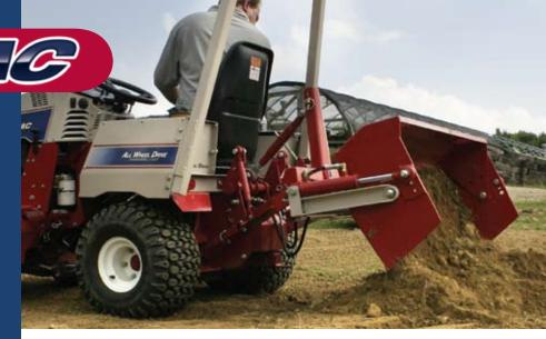
**Connect to the front or rear:** The Ventrac excavator buckets can be mounted to the rear of Ventrac 4000 series tractors equipped with a three point hitch and 3-N-1 Adapter.
